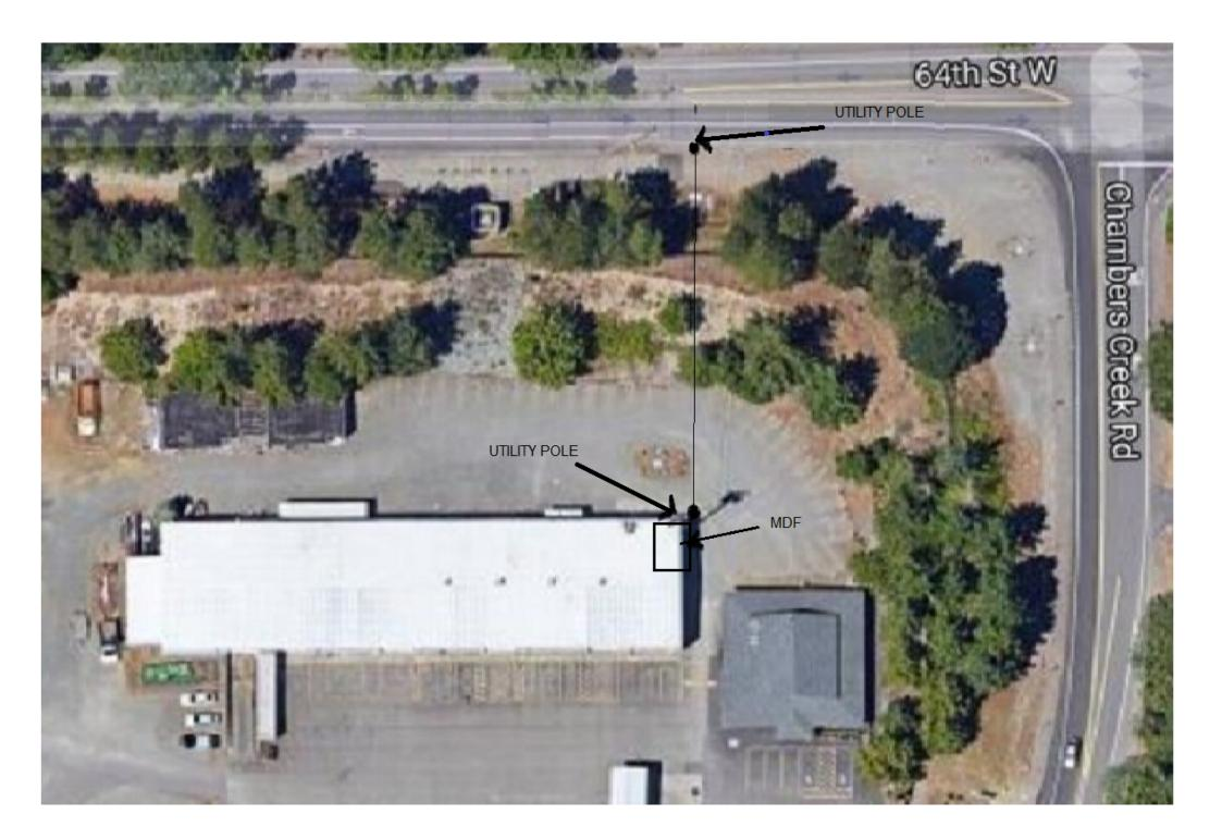
Utilities are provided via aerial connection. There is no visible open conduit from Utility Pole into MDF. Fiber should be terminated in wall mounted cabinet in MDF.
